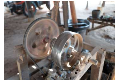
An individual village miller makes sesame and groundnut oil for himself and other villagers using a traditional milling machine. The shed containing the machine sits in the home compound and used to be ox-powered, but was converted to electric motor.
